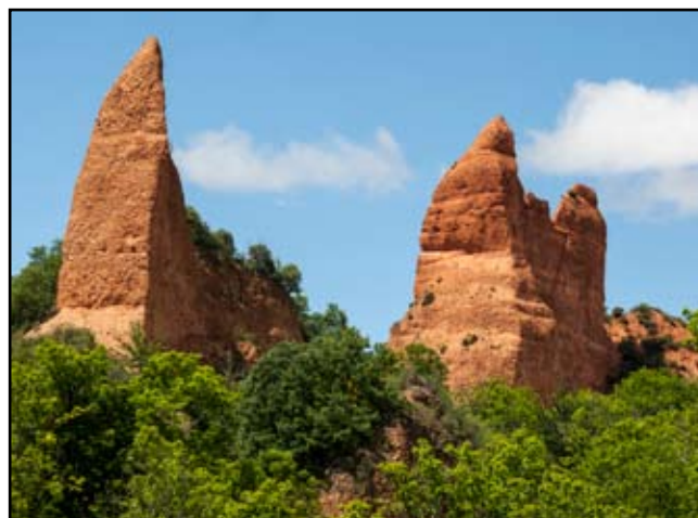
Towers of red conglomerate are remnants where gold values in the basal ore beds were too low to be worth working; their vertical walls were created by the multi-level mining.
